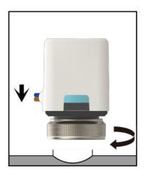
Rotate the nut clockwise and install it on the valve
