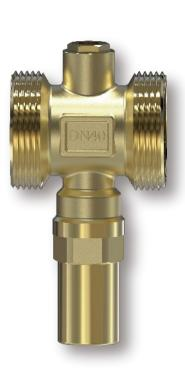
Anti-freeze valves are used in closed circulation system of heat pump, avoiding the freezing of water in the pipes and subsequent damage to the pipe and valve in case of unexpected power outages or system failures, When the water temperature in the system drops below 3°C, the anti-freeze valve automatically opens to drain the circulating water from the pipes.
