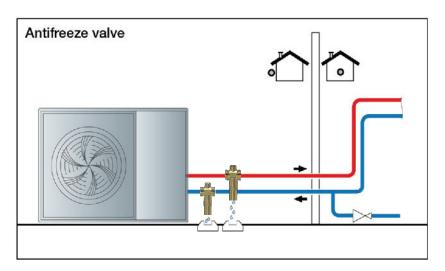
The outlet of the anti-freeze valve should be at least 15cm above the ground level to prevent ice accumulation from obstructing the outlet.
