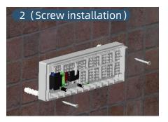
Mark the two fixing holes for the basis and drill them. The basis must horizontally aligned. Install the basis with dowels and screws (2 units M4) depending on the condition of the wall.
