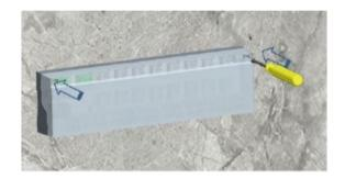
Loosen the casing cover at both latching points with a screwdriver and remove it.
