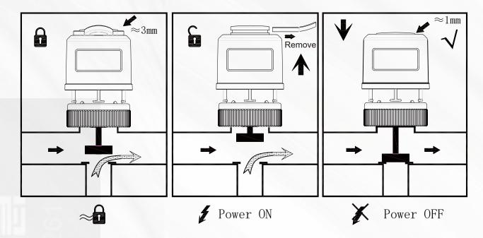
Normally Closed (Initial Installation Power On/Off Indication)
