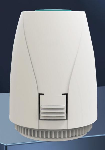
Thermal actuators are mainly used in oor heating systems to control closing and opening of the valves. It is specically applied to electric drive part of the branch manifold valve, small valve and dynamic balance valve. No noise, fast installation and easy disassembly
